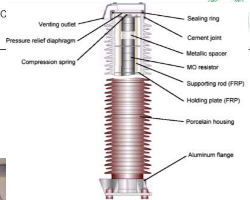
Fig. 8: Cross-sectional drawing of the unit of a porcelain housed MO arrester
